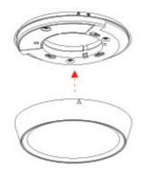
**Step 6** Align the luminaire to the base plate.
