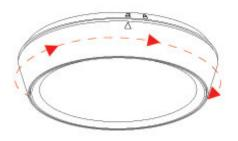
**Step 7** Twist the luminaire clockwise to lock into position.
