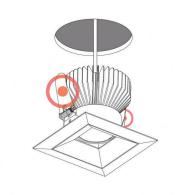
**Step 3**Pull back the springs and insert the luminaire into the ceiling cavity.
