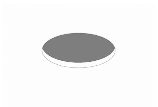
**Step 1**Using a 92mm hole saw, cut a hole in the ceiling at the desired location.
